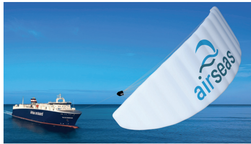
The Seawing's 500 m cable allows a pull angle of 30°, with the kite high enough to exploit faster winds.
